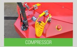
With the optional compressor, the air brakes of the trailer can be quickly released. In addition, a special braking system is available with which the brakes of the trailer can be used to generate extra braking power on slopes or a loading dock.
