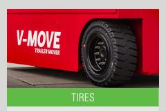
The special solid tires provide maximum traction on slippery and / or wet surfaces.
