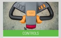
The V-move Trailer Mover is easy to operate with the ergonomic tiller head. Standard equipped with stepless drive control, speed switch and anti-collision protection.
